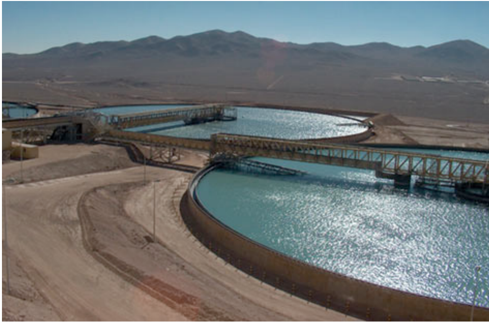
FIGURE 1. Thickeners at Escondida Copper Mine, Chile, whose purpose is the recovery of water from tailings suspensions after flotation.
